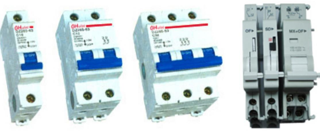
**Applicable Range** HH65-63 miniature circuit breaker is designed for overload and short circuit protections with current limited high breaking capacity, mainly applied to AC 50/60Hz circuit with rated voltage 400V or less and rated current 63A or less. HH65 series miniature circuit breakers (hereinafter called the breakers) are composed of moulded case, operating mechanism, contact, arc-extinguishing system, tripping mechanism etc.
